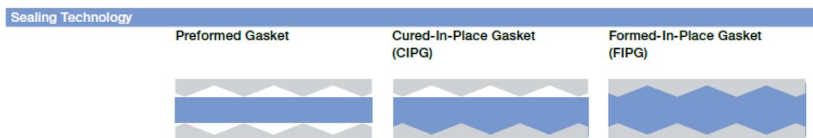
**Figure 9 Comparison of conventional preformed gaskets with cure in place and form in place gaskets.**
