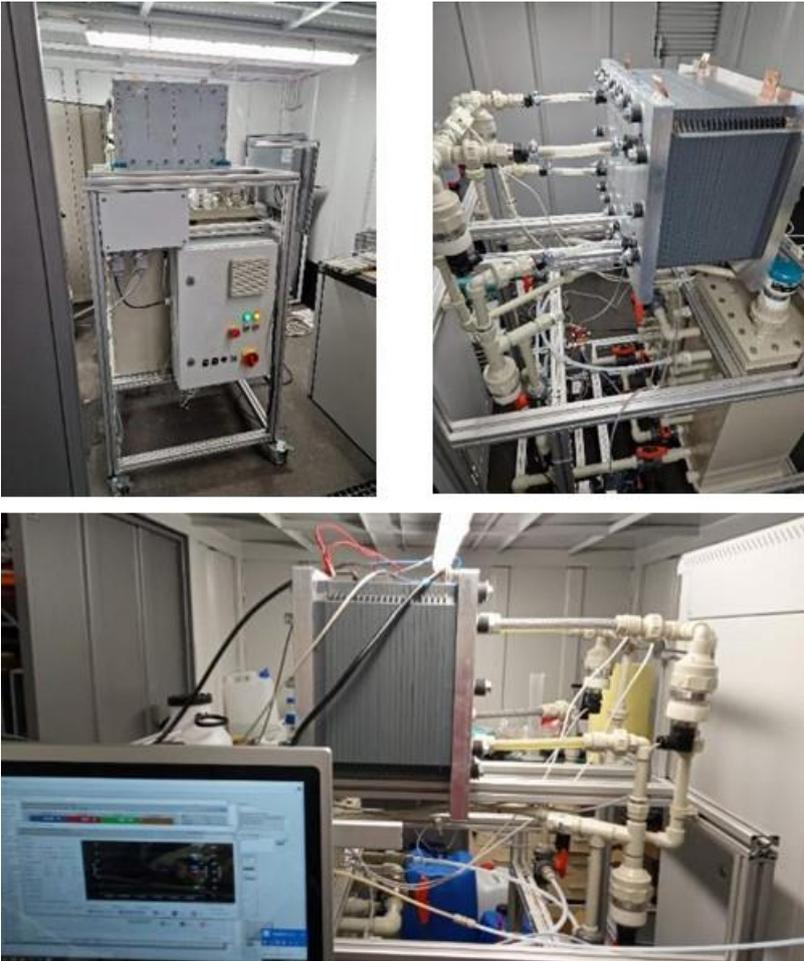
Figure 3 Large system for testing of 20-cell stack.
